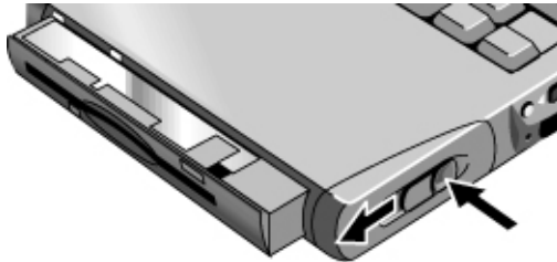
Figure 2-3. Removing a Module
